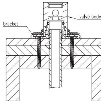
3. Before attach the screws provided to the wood blocking, drill four holes into wall materials by passing through the slots of bracket. Attach with minimum 1 3/4" long screws the bracket through the wall surface into the wood blocking.
