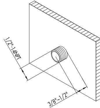
1. RUN 1/2" IPS/NPT threaded stub out pipe through center of blocking board; length of stub out to allow 1/2" to extend beyond the FINISHED WALL SURFACE.
