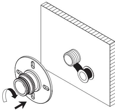
2. After the wall is finished, install the mounting bracket. Apply pipe tape to the threads of stub-out pipe. Screw on the wall mount bracket clockwise.
