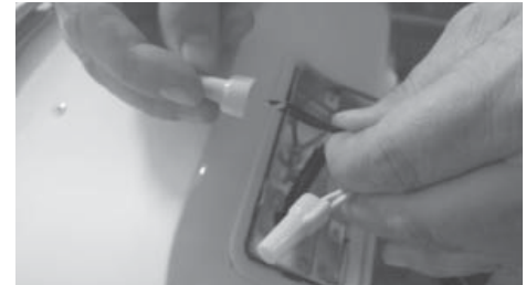
Figure 18 - Connecting the electrical wires.
