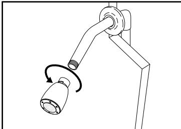
**1. Remove existing shower head.** Turn the existing shower head counter-clockwise with adjustable wrench or pliers. Use care not to unscrew the shower arm; hold the shower arm secure. **NOTE:** If your shower arm has a ball on the end of it, it will not work with this shower unit and will need to be replaced with a standard shower arm.
