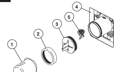
**Turn off water supplies.** Remove cover (1), bonnet nut (2) and test cap (3) from the body. Place a bucket or small container over the front of the valve body and slowly open the water supplies to flush any debris from the supply lines before installing the cartridge. Turn the water supplies back off. If this is not a thin wall mounting, the entire plasterguard (4) may be removed. If screen (5) is in place, remove before installing cartridge.
