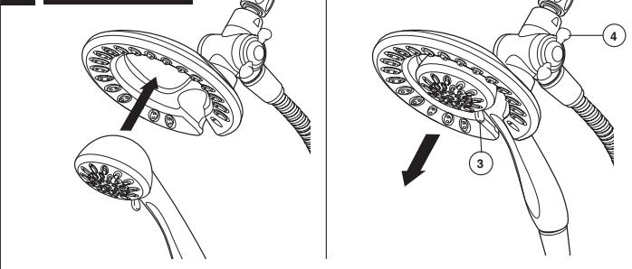
**B. 58045:** To combine the two showers, insert the top tab (1) on the handshower into the slot (2) of the showerhead. Push the handshower into the showerhead until the two parts snap together.
