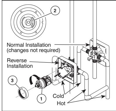
For back to back or reverse installations (hot on right and cold on left): Rotate cartridge (1) so the words "HOT SIDE" (2) appear on the right. Install the cartridge making sure that the key is fully engaged with the slot in the brass body (See step C). Slide bonnet nut (3) over the cartridge and thread onto the body. Hand tighten securely.
