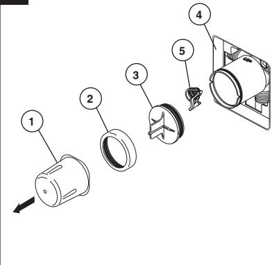
**Turn off water supplies.** Remove cover (1), bonnet nut (2) and test cap (3) from the body. If this is not a thin wall mounting, the entire plasterguard (4) may be removed. If screen (5) is in place, remove before installing cartridge.
