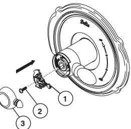
Secure temperature control knob (1) with screw (2). snap on temperature control cover (3) with side snaps onto knob (1).
