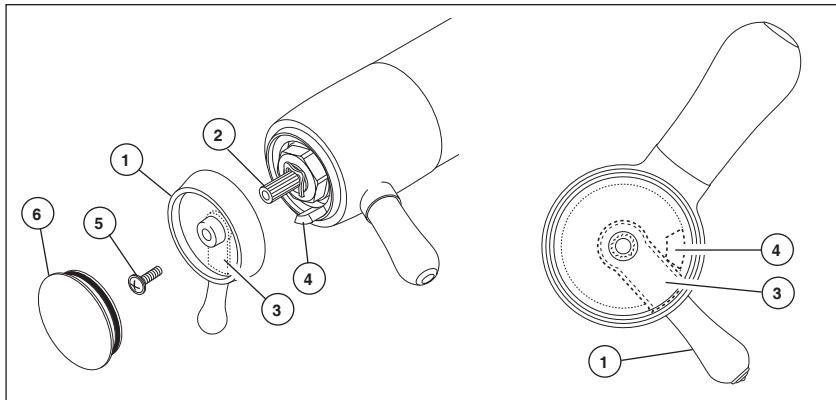
**Adjust temperature limit stop!** Turn on water supplies; LET THE WATER RUN AT BOTH FULL HOT AND FULL COLD TO ENSURE THE WATER IS RUNNING AS HOT/COLD AS POSSIBLE. Place a thermometer in a plastic tumbler, and hold the tumbler in the water stream. Place the temperature knob (1) onto the splines (2), then rotate the temperature knob until you achieve your maximum
