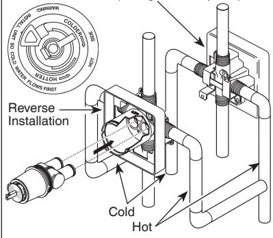
For back to back or reverse installations (hot on right and cold on left) insert the cartridge with the "hot side" on the right. If you are not making a reverse or back to back installation skip this step and continue with step 1C.
