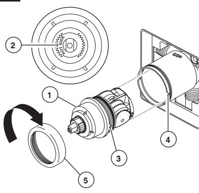
Rotate cartridge (1) so the words "HOT SIDE" (2) appear on the left. Insert cartridge assembly into valve body. Make sure the key (3) on the cartridge is fully engaged with the slot in the brass body (4). Slide bonnet nut (5) over the cartridge and thread onto the body. Hand tighten securely.
