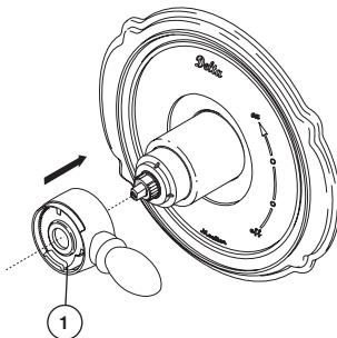
Install volume control handle (1) with lever to the right, then turn to the on position.
