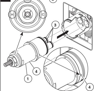
Rotate the cartridge (1) so the word "UP" (2) appears on the top. The "H" must be on the hot side and the "C" must be on the cold side. Add silicone lube to the three o-rings (3) shown above to make the cartridge easier to install and remove from the valve body. Insert cartridge into valve body as shown. Ensure the keys on the body are fully engaged with the slots in the body (4).
