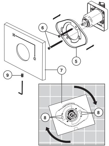
Secure the escutcheon (1) and backplate (2) (if your model has one) to the bracket (3) using the 2 screws provided (4). Do not overtighten escutcheon screws. **If you are installing the Cassidy models T17097, T17297 & T17497:** Thread the cover (5) onto the escutcheon (1).
