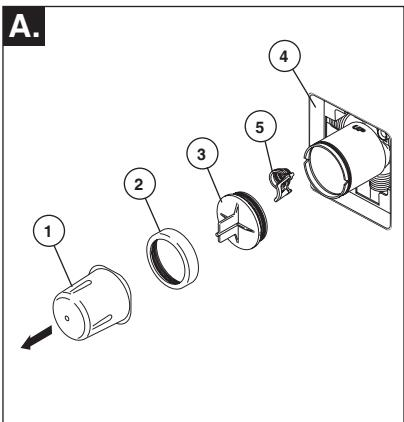
**Turn off water supplies.** Remove cover (1), bonnet nut (2) and test cap (3) from the body. If this is not a thin wall mounting, the entire plasterguard (4) may be removed. If screen (5) is in place, remove before installing cartridge.
