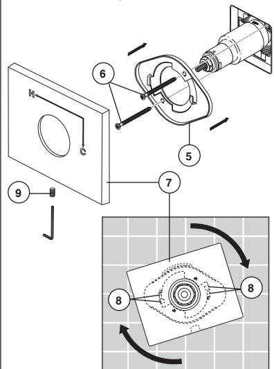
Secure the escutcheon (1) to the bracket (2) with the 2 screws provided (3). Do not overtighten escutcheon screws.
