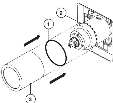
Slide O-ring (1) over cartridge and the bonnet nut (2). The O-ring, which acts as a spacer to steady the sleeve, should rest behind the bonnet nut. Slide the sleeve (3) over the cartridge, body and O-ring. Ensure sleeve is properly positioned over the front of cartridge.
