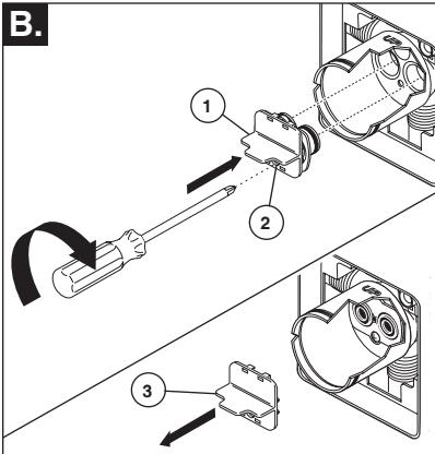
Insert adapter assembly (1) into valve body. Make sure the adapter assembly is correctly positioned and is pressed all the way down inside body. Secure adapter with the screw (2) provided in the adapter assembly. Remove the retainer (3) from the adapter.
