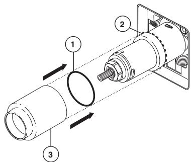
Slide O-ring (1) over cartridge and the bonnet nut (2). The O-ring, which acts as a spacer to steady the sleeve, should rest behind the bonnet nut. Slide the sleeve (3) over the cartridge, body and O-ring. Ensure sleeve is properly positioned over the front of cartridge.
