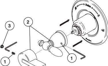
Using an Allen wrench to secure the set screw (1), install the handle (2) onto the stem. Insert plug button (3) (if your model has one) into set screw hole.
