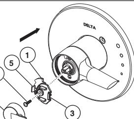
Secure temperature control knob (1) with screw (2). Hook (3) front of temperature control cover (4) onto knob (1) before engaging rear snap (5).
