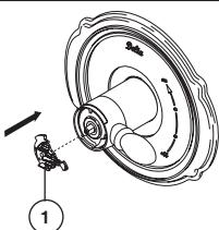
Place the temperature control knob (1) on volume handle and rotate to the mixed position (if required). DO NOT SECURE WITH SCREW. Turn on water supplies; let the water run until both hot and cold water is as hot/cold as possible. Place thermometer in a plastic tumbler, and hold the tumbler in the water stream. Record the temperature reading.
