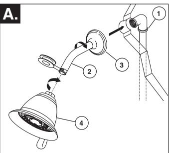
**FOR SHOWERHEAD INSTALLATION:** Connect top outlet (1) to shower arm (2) with proper fittings. To prevent damage to finish on shower arm, insert wall end of shower arm into shower flange (3) before screwing arm into riser connection. Thread showerhead (4) onto shower arm. Apply plumber tape to pipe threads on both ends. Do not overtighten showerhead.
