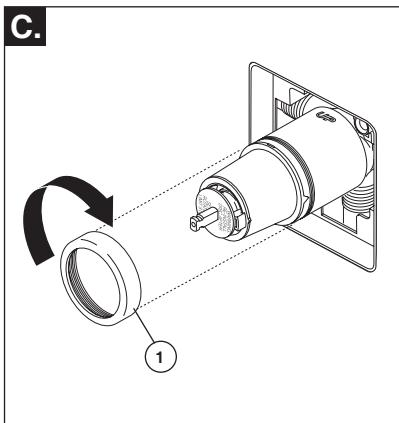
Slide bonnet nut (1) over the cartridge and thread onto the body. Hand tighten securely.
