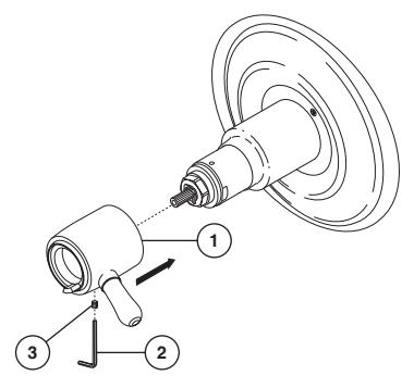
Install volume control handle (1) with lever to the right, using an Allen wrench (2) to secure with the set screw (3).
