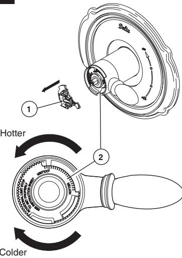
If the water temperature is above 120°F, remove the temperature control knob (1) and rotate the limit stop (2) clockwise one tooth for every 4°F - 6°F (approximate) change in temperature. If water temperature is cooler than desired, rotate the limit stop counterclockwise.
