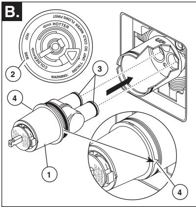
Rotate the cartridge (1) so the words "hot side" (2) appear on the left. Insert cartridge into valve body as shown. Make sure the cartridge tubes and O-rings (3) are properly seated in holes at the base of the body. Ensure the keys on the body are fully engaged with the slots in the body (4).
