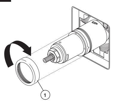
Slide bonnet nut (1) over the cartridge and thread onto the body. Hand tighten securely.
