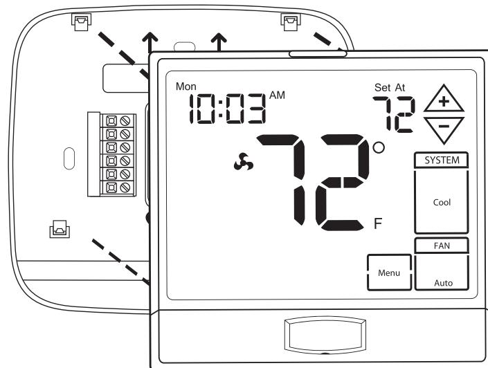
Align the 4 tabs on the subbase with corresponding slots on the back of the thermostat, then push gently until the thermostat snaps in place.
