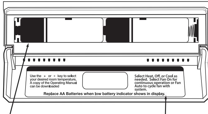
Insert 2 AA Alkaline batteries (included). High quality alkaline batteries are recommended.
