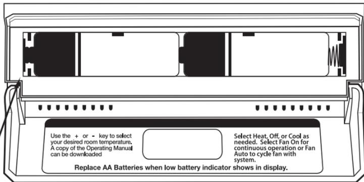
Insert 2 AA Alkaline batteries (included). High quality alkaline batteries are recommended.
