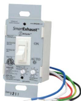
There are only two settings on the FT622: VENTILATION and DELAY. The VENTILATION setting allows the user to set the number of minutes per hour the fan should run. The DELAY setting allows the user to set the number of minutes the fan should run after the bathroom light has been turned off. The DELAY setting provides additional run time for the fan to complete the remaining necessary ventilation after use.
