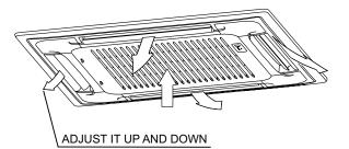
While this function is set, the swing fan of indoor unit runs; otherwise, the swing fan doesn't run. The swing scale of every side is 30°. When the air conditioner isn't in operation (including when "TIMER ON" is set), the SWING button will be disabled.
