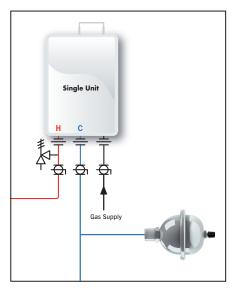
ZEP-1 can be installed below the isolation kit or anywhere on the cold water supply line between the heater and the check valve.
