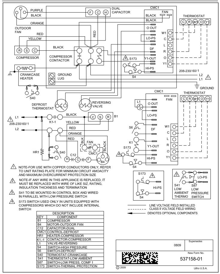
Figure 4. 14 SEER Wiring Diagram
