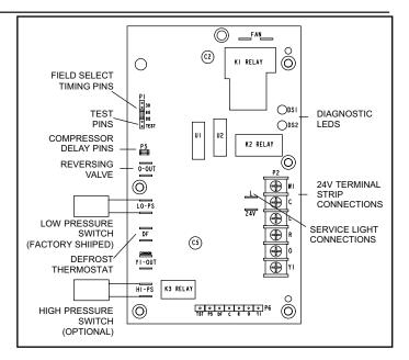
Figure 3. Outdoor Unit Defrost Control Board
