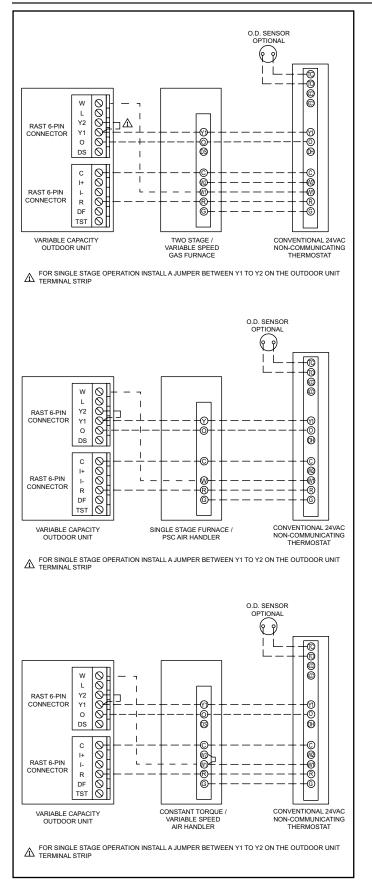
Figure 9. Conventional 24VAC Cooling Non-Communicating Thermostat Wiring - Single Stage
