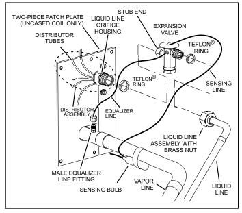
Figure 4. Remove Expansion Valve (Uncased Coil Shown)
