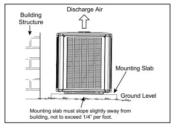
Figure 1. Slab Mounting
