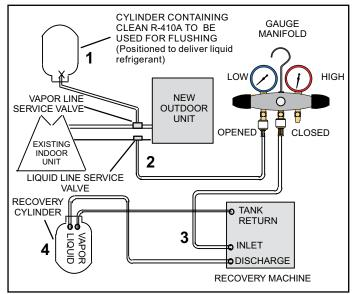
Figure 5. Connecting Gauges
