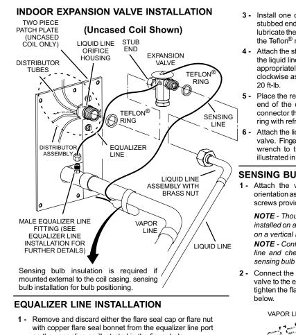
on the vapor line as illustrated in the figure below.
